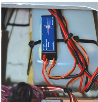
Installation of such a small unit is simplicity itself, in this case being servo taped to a small mounting plate, which is cable-tied to the fuel tank
