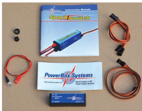
SparkSwitch set contents include the main electronic switch/regulator, leads, LED and manual. The switch/regulator is extremely compact and light, the sockets for the various leads are clearly marked
