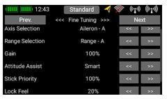
At **SELECT axes** you select the axis which is to be adjusted. At **Select range** you choose the range you wish to adjust. The two ranges can be used to set up two different settings, either of which can be selected in flight using a switch. **Range A** should be selected for gain values between 0% and +100%, while **Range B** runs from 0% to -100%. At 0% the iGyro is completely disabled.
