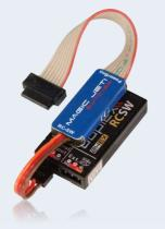
Insert the Bind plug in the RCSW, then connect the **Magic Jeti Switch** to the **PowerBox**. Navigate through your transmitter menu as follows:
