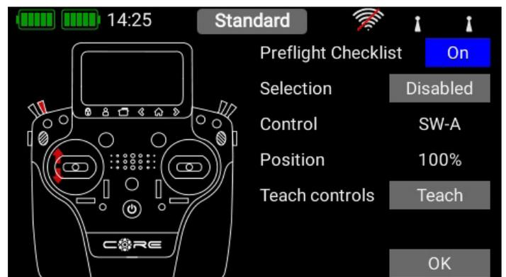
If you switch on or change models and the selected transmitter controls are not in the correct position, then the screen looks like this:
