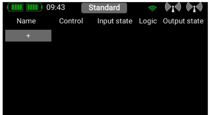
Select the **Virtual Switch** button in the menu, then press **+** to set up a new virtual switch. You can rename the virtual **switch** by pressing the switch button. As you can see, this field includes a small triangle at top right. This means that a function can be selected here by holding your finger on it. In this case the virtual switch can be erased again by holding your finger on the switch button.
