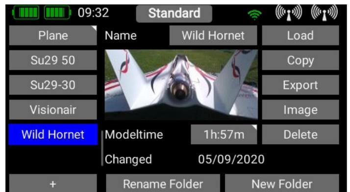
To create a new model, briefly touch the + button at the bottom of the screen. Assign a name to your model, and confirm your choice with OK. You will now see the Select screen for the model type. At this point you can select the appropriate model type, with the additional options of delta wing and V-tail.
