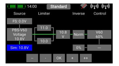
If the telemetry control is above the set value of 11.0V, 0% is added to the throttle servo, i.e. the throttle channel behaves in the usual way.
