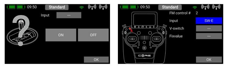
At this point you can select the appropriate transmitter control. If you select a switch, you can activate one or two switch positions. If you choose a linear control, you can set the switching threshold and hysteresis here. If you have already set up virtual switches, please note that you can also use these for selecting the flight mode.
