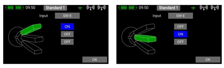
When you have set up multiple flight modes, you will see green dashes in the Flight Mode tree which indicate which flight mode is currently active. You can now select various settings for the different flight modes in the Transmitter Control, Trim and Mixer menus after selecting the Single setting at Flight Mode.
