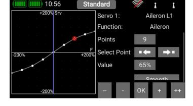
Here you will find the assigned servos again. Up to eight servos can be assigned to each function. As already mentioned in the **Assistant**, the travel and end-points of each servo can be adjusted separately here. Any adjustments you make to a servo at this point have no influence on the settings of the same servo if it is also assigned to another function. This provides a simple means of mixing in aircraft with multi-flap wings, delta wings and V-tails.
