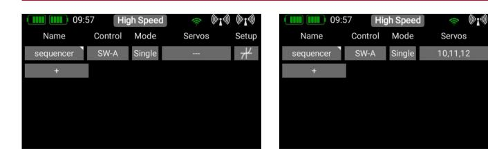
At the Overview screen press **Setup** to set the travel points. You will see the next screen display shown here. The first servo is marked, and the sequence **Forward** and **Reverse** is displayed. The standard run time is 6.0 seconds, and the two travel points are set at ±20%.
