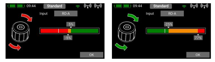
The two switching points can now be placed in any position you like by moving them with your finger. The red area indicates the "**Off**" state; the green area the "**On**" state. The orange area indicates "**hysteresis**", i.e. the area in which no switching takes place.
