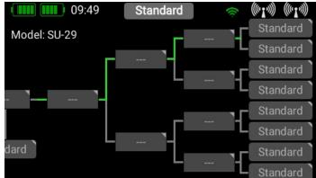
The most important thing to know at this point is that the **CORE** prioritizes the flight modes. Priority runs from left to right, i.e. the flight modes in the left-hand tree diagram have the highest priority, and those on the right the lowest priority. Even when the flight mode structure is complex, this means that you can, for example, overrule all other switch positions with a single switch, returning you very quickly to "normal" flight mode.
