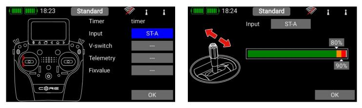
The two switching points can now be placed in any position you like by moving them with your finger. The red area indicates the "**Off**" state, the green area the "**On**" state. The orange area indicates "**hysteresis**", i.e., the area in which no switching takes place.
