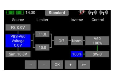
To conclude our example, you can now see how the telemetry control is set in such a way that motor power is reduced by 50% when battery voltage falls to 11.0V.
