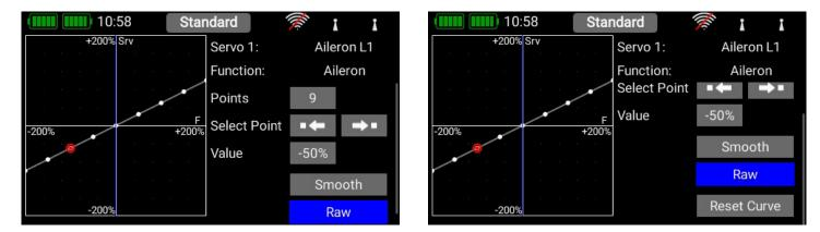
This is the procedure: use the arrow buttons to select the point you wish to adjust. Briefly press the displayed setting at **Value**, then adjust the servo for this position. The **Smooth button** can be used to even out the course of the curve. Right at the bottom you will find a **Reset button** which sets the curve back to a straight line. Once you have set the desired curve, return to the Servo Curve menu, where you will find three Preview buttons:
