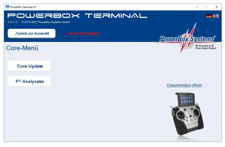
Insert a USB stick in your PC, and follow the on-screen instructions. The USB stick will now be formatted, and all the essential data copied onto it. Once that is finished, switch your CORE transmitter on and wait until it has booted up. Now insert the USB stick in the CORE transmitter, move to the **Settings > System > Software**.
