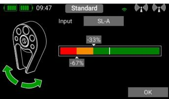
When you have selected a linear transmitter the two switching points can be placed in any position you like by moving them with your finger. The red area indicates the "Off" state; the green area the "On" state. The orange area indicates "hysteresis", i.e. the area in which no switching takes place. You can very easily reverse the "Off" state and the "On" state by moving one of the two switching point sliders in front of or behind the other.
