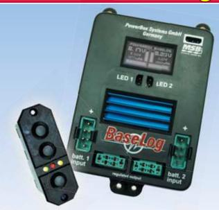
Universal power supply system for RC models with redundant electronic components, info-display, menu-based programming and telemetry link
