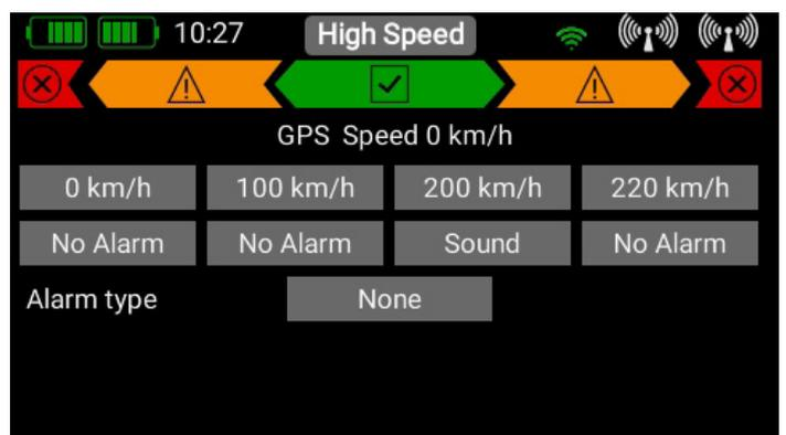
The final step is to select the type of warning you want. In our example a warning tone is set to be generated at 200 km/h, while a spoken message is generated at 220 km/h.
