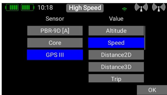
The left-hand column shows all the connected sensors, while the right-hand column shows all the values which these sensors supply. The **P<sup>2</sup>BUS** is an in-house development, and is capable of transmitting up to **255 sensors each with 32 individual values** – and at a speed of up to **800 values per second!**
