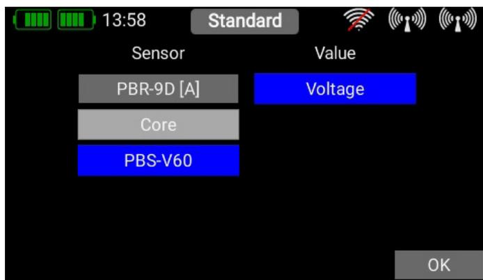
In this example the **PBS-V60** voltage sensor is to be used to reduce motor power if the voltage of the flight battery falls to a dangerous level. You can rename the telemetry control under the **Name** field.
