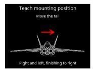
This is accomplished by moving the aircraft in the directions shown in the graphic display: first move the tail of the aircraft up and down two or three times. You will see that the elevators follow this movement every time - the direction of effect is not important at this stage.
