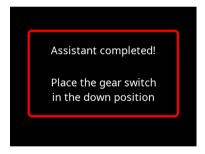
The Assistant now opens all the wheel doors and moves the undercarriage to the **Extended** position. At this point you can check the operation of the sequencer by operating the retract switch on the transmitter. If you find a problem - perhaps the pause between the undercarriage and the wheel doors is too short - you just select the Assistant again, and change the appropriate setting. There is no need to re-adjust the wheel door positions.
