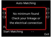
A matching process for three servos takes about 30-40 seconds. You can follow the current consumption directly on the screen. When the matching is finished, use the transmitter stick to run the servos to all five points. A quiet buzz from the servos in one or other position is normal. If the buzzing stops when you touch the control surface lightly with your finger, then this shows that the matching process has worked accurately.
