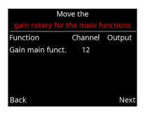
You need to assign a channel with +/-100% travel to a rotary control at the transmitter. Even if you have not connected an iGyroSat, this action is recommended as it will make it easier to retro-fit the gyro.
