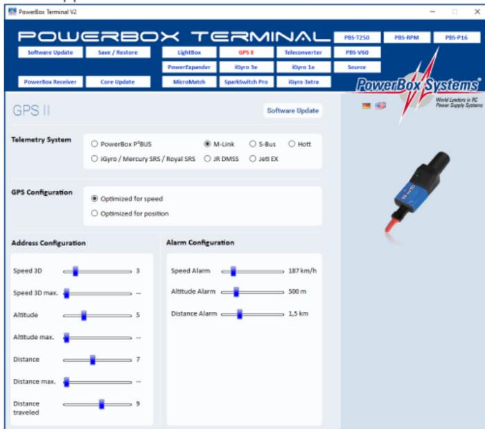
The first step here is to select the telemetry system you wish to use. The lower part of the screen displays various set-up facilities which vary according to the telemetry system you select.
