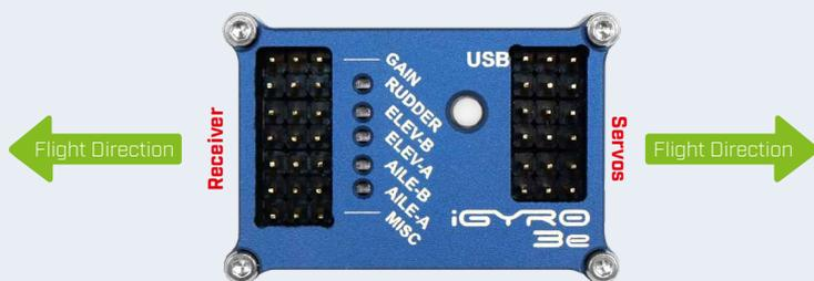
2. Connect the patch-leads to the receiver, and connect the servos.
