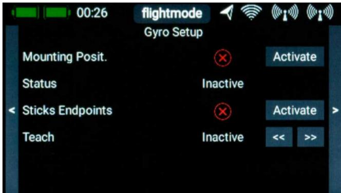
The installed position of the **iGyro SAT** and the stick zero and end-points are established at this screen.
