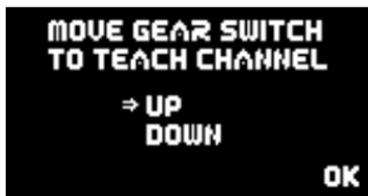
Operate the appropriate transmitter switch, and the **PowerBox** automatically detects it as the switch which you have assigned to the retract system. The on-screen arrows should now be located in front of **UP/DOWN**. If you find that your retract switch works in the wrong "sense" (direction), correct it by reversing that output at the transmitter. Press the SET button again to proceed.
