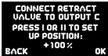
The undercarriage should now retract. If not, hold button I pressed in until the valve is triggered, and the undercarriage retracts. Press the SET button to move on to the next stage of the procedure:
