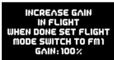
Launch the model and fly at half-throttle parallel with the landing strip. Increase gyro gain until the aircraft just starts to oscillate around one axis. At this point reduce gain slightly until the model shows no sign of oscillating in **any** speed range.
