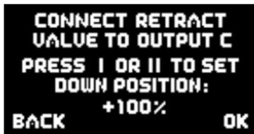
Connect your retract system valve to output **C**. One of the following will now occur, depending on the way your valve is programmed:
