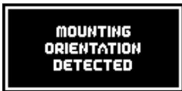
You can install the **Mercury SRS** in any position, provided that the case is at right-angles (90°) to the fuselage centreline.
