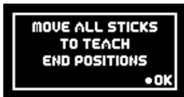
The **Mercury SRS** carries out a self-calibration of the gyro sensors, and resets the maximum permitted control surface travels. In the next screen display you are requested to move all the transmitter sticks to both end-points. When you have done this, confirm by selecting **OK**.
