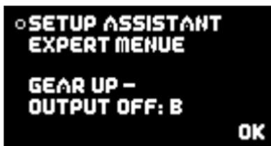
The **SETUP ASSISTANT** is a function in the **Cockpit** which has been included since software version V15; it makes the task of programming the actual door sequencer function considerably easier.
