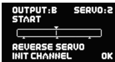
To ensure accurate servo matching, the output to be adjusted must first be initialised. Leave the associated transmitter stick at centre. Move the cursor to **INIT OUTPUT** and press the **SET button**. Now move the transmitter stick to both end-points.
