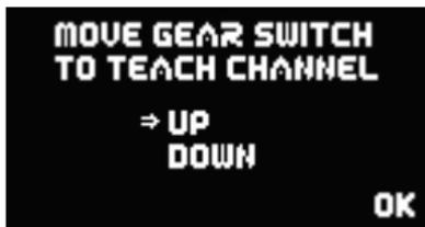
Operate the appropriate transmitter switch, and the **PowerBox** automatically detects it as the switch which you have assigned to the retract system. The on-screen arrows should now be located in front of **UP/DOWN**. If you find
