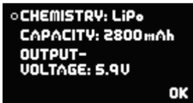
If you wish to change one of the settings, use buttons **I** and **II** to move the cursor to the appropriate menu point, then press the **SET** button to select it (cursor changes to a solid disc). You can now alter the value using buttons **I** and **II**. Once you have selected the desired value, press the **SET** button to confirm it; this saves (stores) the new value. Select the menu point **OK** to return to the main menu.
