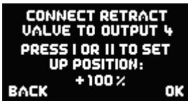
The undercarriage should now retract. If not, hold **button I** pressed in until the valve is triggered, and the undercarriage retracts. Press the **SET button** to move on to the next stage of the procedure.
