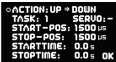
In the Expert Menue, the sequencer does not constrain you to use pre-set modes, forcing you to adopt fixed, pre-determined vectors for retracting and extending the undercarriage.
