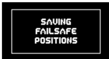
Check the settings by moving all the functions to any "non fail-safe position" at the transmitter - e.g. move throttle to "full-throttle" - then switch the transmitter off. All the outputs which are marked **FS** in the **OUTPUT MAPPING** menu should now move to the previously set positions, whereas all outputs not marked **FS** remain in the last known position.
