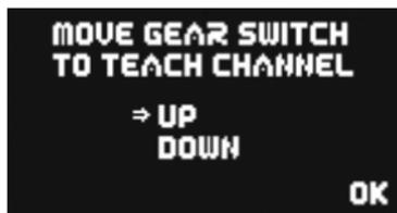
Operate the appropriate transmitter switch, and the **PowerBox** automatically detects it as the switch which you have assigned to the retract system. The on-screen arrows should now be located in front of **UP/DOWN**. If you find that your retract switch works in the wrong “sense” (direction), correct it by reversing that output at the transmitter.
