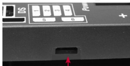
Socket for **USB Interface** and telemetry: P<sup>2</sup>-BUS, M-Link, HoTT and Jeti
