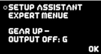
The **SETUP ASSISTANT** is a new function in the **Cockpit SRS** which has been included since software version 15; it makes the task of programming the actual door sequencer function considerably easier.
