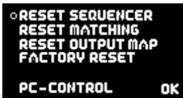
In the interests of safety, the software generates a confirmation query when you select one of the Reset options; the intention is to avoid accidental erasure of data. If you confirm this query, the settings are permanently erased, and cannot be restored.
