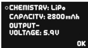
If you wish to change one of the settings, use buttons **I** and **II** to move the cursor to the appropriate menu point, then press the **SET** button to select it (cursor changes to a solid disc). You can now alter the value using buttons **I** and **II**. Once you have selected the desired value, press the **SET** button to confirm it; this saves (stores) the new value. Select the menu point **OK** to return to the main menu.
