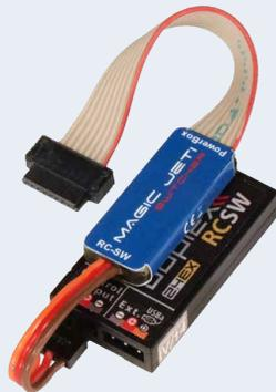
Insert the Bind plug in the RCSW, then connect the **Magic Jeti Switch** to the **PowerBox**. Navigate through your transmitter menu as follows:
