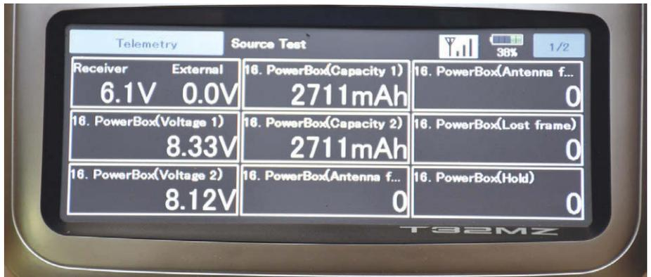
Telemetry display on my Futaba 32MZ transmitter, with data showing for the input voltages of both batteries and their remaining capacities – the remaining fields are for use with different PB units.
