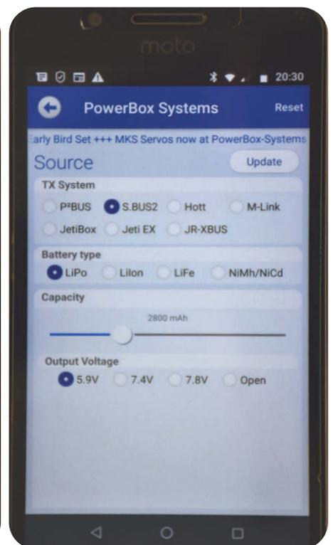
Specific Source screen where Tx operating system, battery type, capacity and output voltage can be set.
