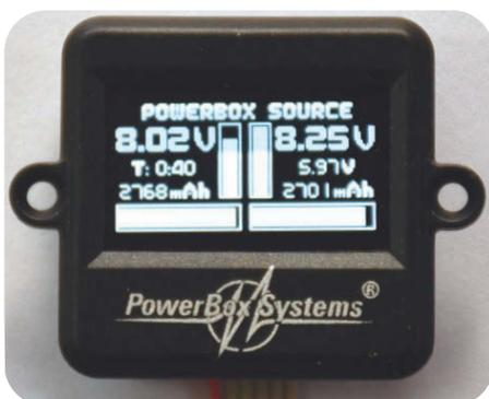
Main screen of the OLED display, showing the input voltages, remaining capacities, output voltage and operating time since reset.
