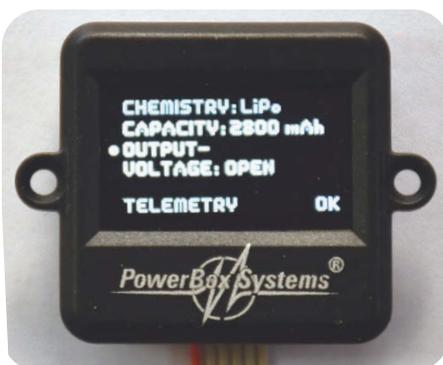
Main set up screen allows all parameters to be selected so that they can be changed or set.
