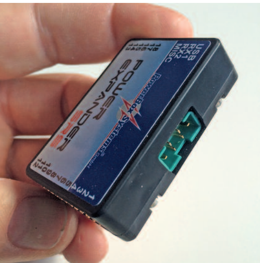
For Futaba users the wait is over. The PowerExpander SRS enables users to exploit all the radio control system's channels even when using small but fully featured receivers. The PowerExpander can be purchased with a Deans connector (top picture) or an MPX connector (bottom picture).
