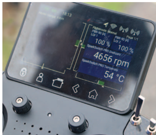
The new PowerBox Core radio displaying the telemetry received from the SparkSwitch Pro, including the head temperature and engine rpm.
