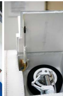
This is looking into the lower fuselage area, near the nose gear retract. Air tanks to each
