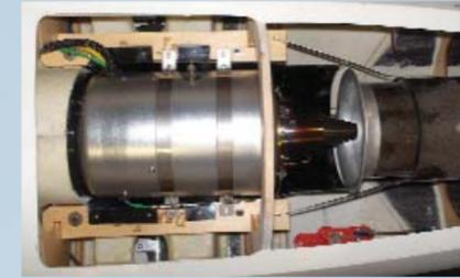
The Super Eagle nestles comfortably in place, just ahead of the supplied tail pipe. All the bulkheads are pre-installed at the factory, just drill holes for the motor mounts and you're done!
