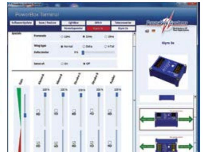
The terminal program accesses several advanced configuration options to optimize your IGyro including individual channel gains and Delta Wing mixing.
