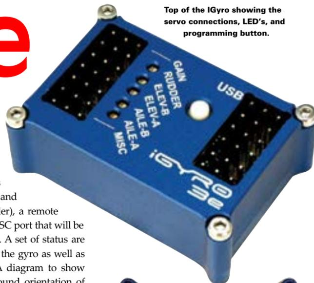
Top of the IGyro showing the servo connections, LED's, and programming button.
