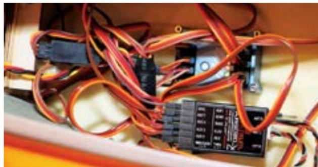
IGyro 3E mounted next to the receiver in my Habu 32x. Before I cleaned up the wiring!
